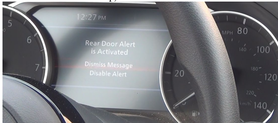
Figure E-6. 2022 Nissan Rogue alert activation visual alert on the instrument panel
