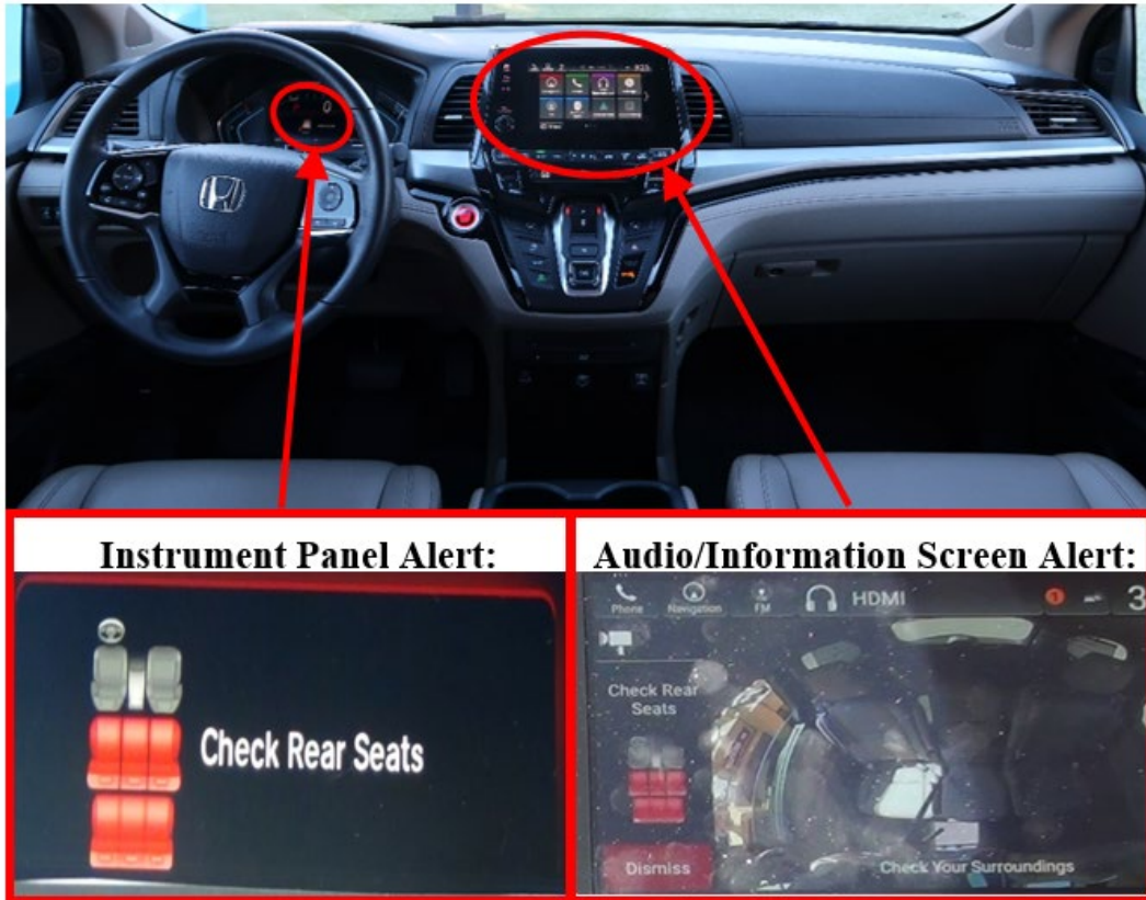
Figure E-8. Honda Odyssey dashboard (top) and close-ups of visual alerts on the instrument panel (bottom left) and audio/information screen (bottom right)
